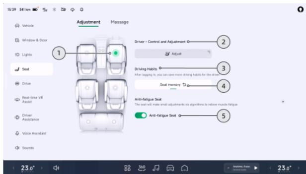
On the “**Seat**→**Adjustment**” interface of the CID, adjust the seat position.
