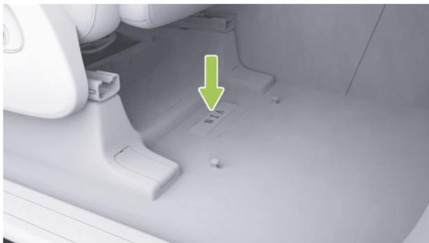
The VIN is stamped under the driver's seat.
