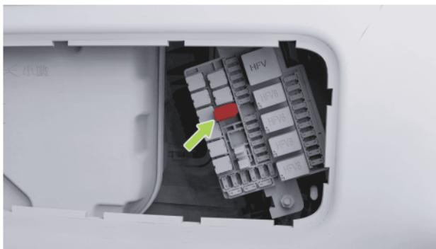
1. Open the trunk and remove the trunk repair cover plate using appropriate tools.
