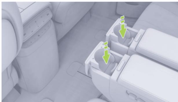
The inner armrest of the second-row seat is equipped with a cup holder to hold drink bottles or cups. Press the switch to eject the cup holder, and push it back to lock it when not in use.
