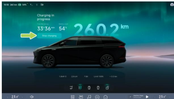
6. If you need to temporarily end the charging process. Click the **“End Charging”** button on the CID. End the charging and confirm at the charging screen that the charging has ended.
