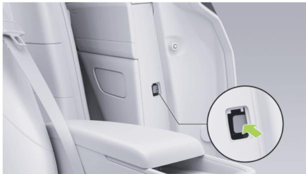
If the Slide door cannot be locked under special circumstances, pry up the side locking panel of the Slide door with a suitable tool, press the internal switch to slide close the Slide door and then the Slide door is locked.
