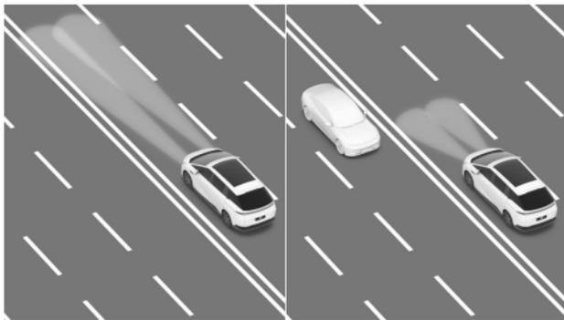
The IHB can automatically switch between high and low beams according to the conditions of
