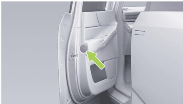
The front passenger door is equipped with push-type umbrella holder.
