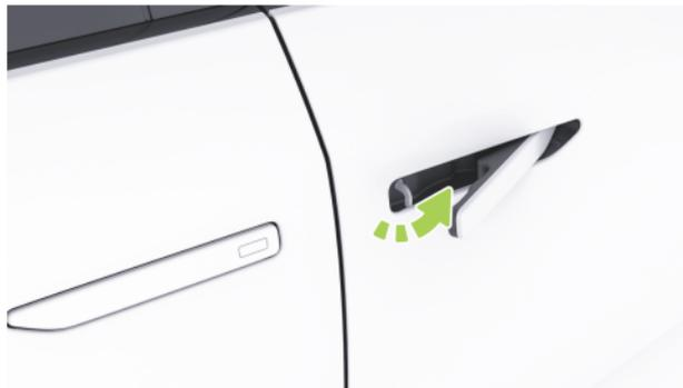
When the vehicle is out of power, press the front end of the concealed door handle and pull it out. Insert the mechanical key into the lock hole, rotate counterclockwise to unlock the door, and then pull the door handle to open the door.
