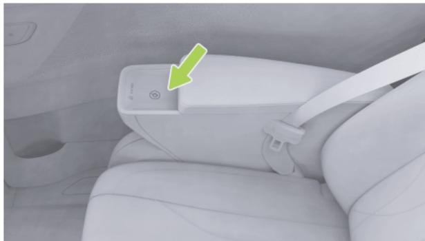
The second-row wireless charging area is located at the outer armrest of the seat. During charging, please face the mobile phone screen upward and slide the mobile phone to the bottom of the charging area along the limit bar.
