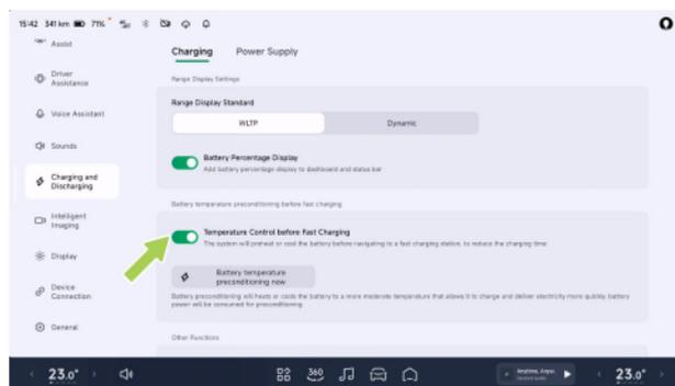
On the “→Charging and Discharging→Charging” interface of the CID, you can turn on “**Temperature Control before Fast Charging**”. When this function is turned on, and the navigation destination is set to a fast-charging station, the vehicle will control the traction battery temperature to the optimal charging range, reducing charging time. Before
