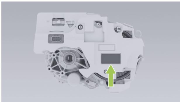
The drive motor model and serial number are displayed on the drive motor housing and the drive motor label.
