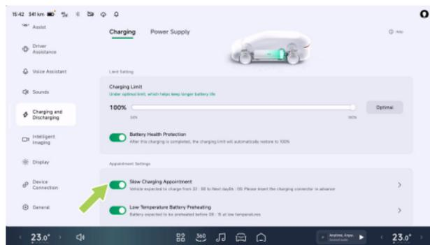
On the “→Charging and Discharging→Charging” interface of the CID, turn on “**Slow Charging Appointment**” to set the start and end times for charging. This allows the use of off-peak electricity rates during nighttime hours, reducing charging costs.
