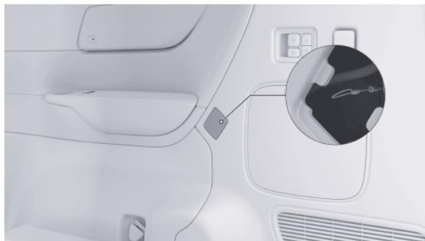
2. Locate the emergency unlock ring of the charging port, pull the ring, unlock and pull out the gun.
