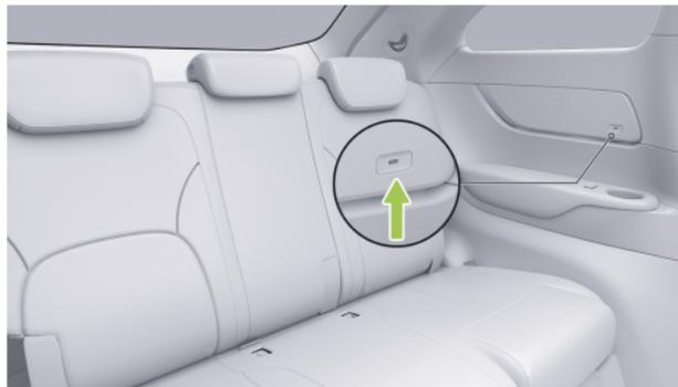
There is one Type-C power port on the third-row left and right side panels respectively, with a maximum power of 15W.
