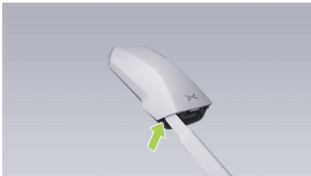
2. Use a suitable tool (slotted screwdriver covered with soft cloth/wrapped with adhesive tape or similar tools) to pry up the left edge and move it towards the center to pry loose the left side of the rear cover.
