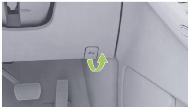
1. Pull the front hood release handle located on the lower right side of the instrument panel twice consecutively to unlock the front hood, which will slightly pop up.
