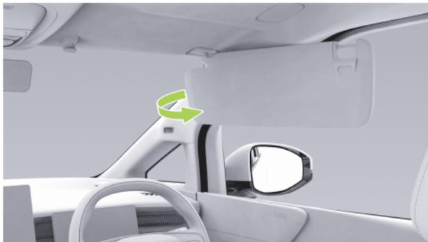
After flipping down the sun visor, take out one end of the sun visor which is close to the interior rearview mirror from the bracket and turn over the sun visor towards the window to block sunlight coming in through the window.
