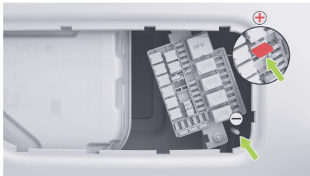
3. Connect one end of the red cable of the 12V charger to the positive terminal clamp point of this vehicle and one end of the black cable to the negative terminal clamp point for charging.
