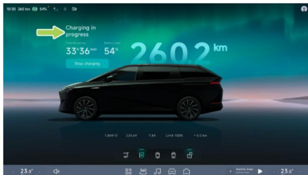
When the vehicle is charging, the message 'Charging/Heating Up' is displayed on the CID, do not pull the gun at this time, as personal injury may result. To end charging early, You must first click on "End Charging" in the CID. The
