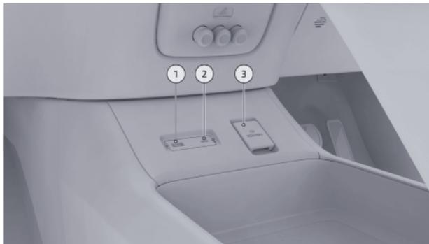
1. USB media source port: It is used for data transmission\*(if applicable), microphone, game controller, etc.
