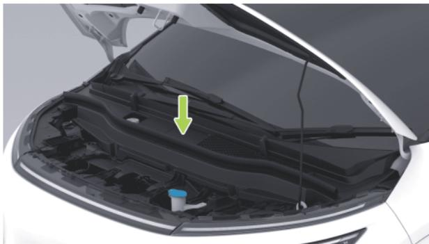
1. Remove the access cover plate with a proper tool to access the coolant reservoir.
