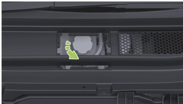
3. unscrew and remove the cap, and add the coolant.
