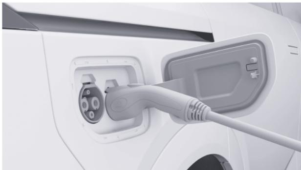
4. Remove the charger gun protective cap and insert the charger gun straight into place, keeping the charging harness loose and hanging naturally.
