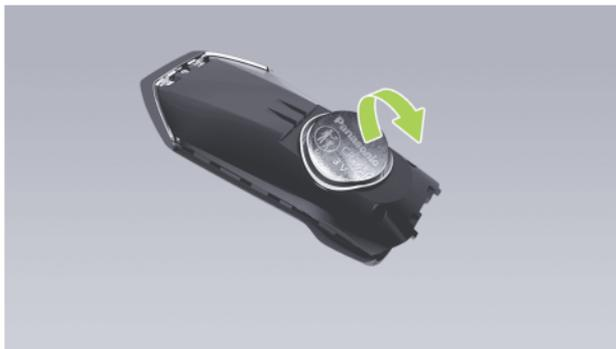
5. Replace the battery. Battery model: CR2450. Make sure that the "+" (positive pole) of the battery faces upward during installation.
