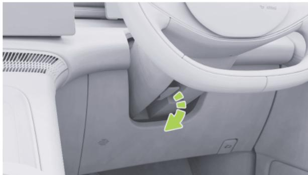
1. Pull the steering wheel unlocking handle downward to unlock the steering wheel.
