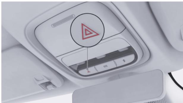
In case of emergency while driving, press the hazard warning light switch to activate the hazard warning light. The turn signal will flash. Press the switch again to deactivate the hazard warning light.
