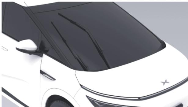
On the “
