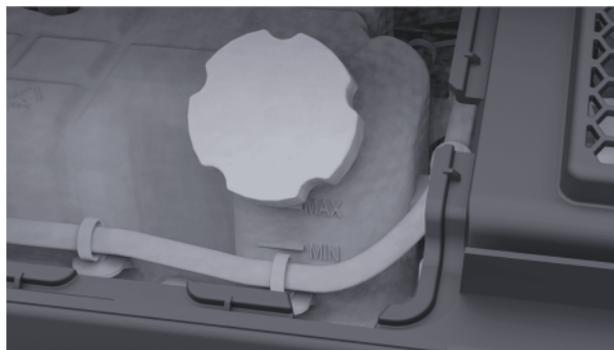
Check the level mark on the side of the coolant reservoir:
