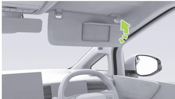
Both driver's and front passenger's sun visors are equipped with vanity mirrors. The vanity mirror light will turn on automatically when the sun visor is flipped down and the vanity mirror cover is lifted, and turn off when the vanity mirror cover is closed.
