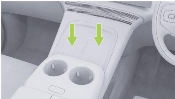
The front-row wireless charging area is located in the front of the console. During charging, please face the mobile phone screen upward and slide the mobile phone to the bottom of the charging area along the limit bar, which is conducive to inductive charging and heat dissipation of the mobile phone. During charging, “Qi” is displayed on the CID.
