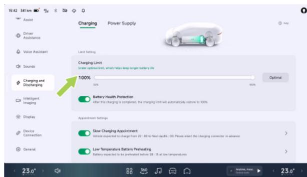
On the “→Charging and Discharging→Charging” interface of the CID, you can set “Charging Limit”, and the charging will automatically end when the set limit is reached.
