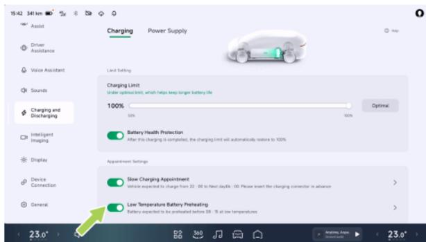
On the “→**Charging and Discharging**→**Charging**” interface of the CID, you can set the preheating start time.
