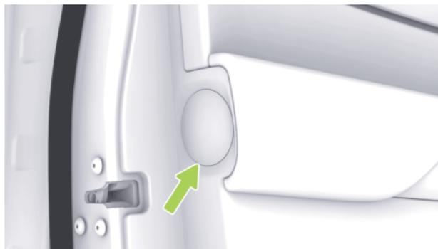
After prying off the umbrella holder cover with a suitable tool (key card covered by soft cloth/wrapped in adhesive tape or similar), the umbrella can be stored or taken out:
