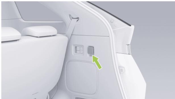
The trunk is equipped with a 12V power port, with a maximum power of 180W.
