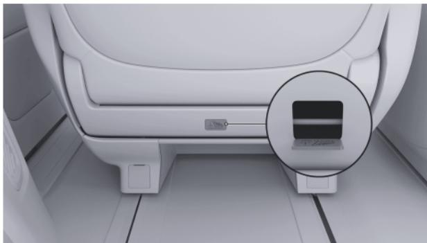
Second row seat: Pass the top fixing belt of the child safety seat through the headrest and pull it to the rear of the backrest. Pry up the anchoring point cover plate with a suitable tool, connect the hook and loop of the fixing belt to the anchoring point, and tighten the fixing belt.
