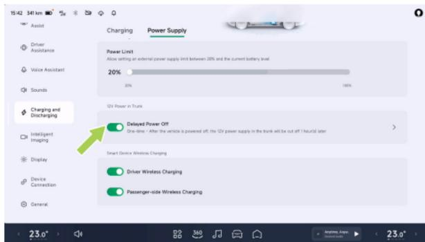
On the “**Charging and Discharging**→**Power Supply**” interface of the CID, after turning on “**Delayed Power Off**”, you can set the delayed power-off time of the trunk 12V power supply after the vehicle is powered off.
