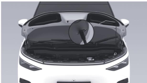
2. Lift the front hood to its limit position, remove the support rod from the fixing groove, and secure it into the opening on the hood.
