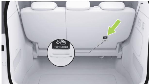
Third row right seat: Pass the top fixing belt of the child safety seat through the headrest and pull it to the rear of the backrest. Connect the hook and loop of the fixing belt to the anchoring point, and tighten the fixing belt.
