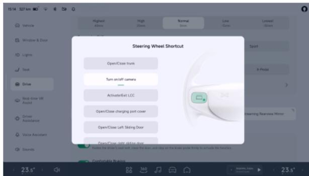
By pressing and holding the steering wheel shortcut key, or on the “**Drive**→**Steering wheel Shortcut**” interface of the CID, you can set the steering wheel shortcut key function.
