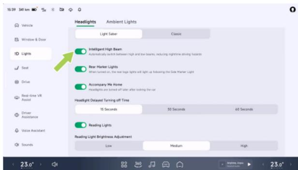
On the “**☰→Lights→Headlights**” interface of the CID, you can turn on/off “**Intelligent High Beam**”.
