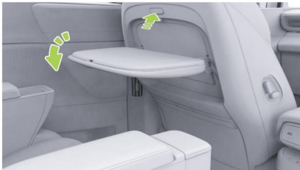
There is a foldable tray on the back of the front seat, which can be unfolded by pressing the switch, and folded when not in use.
