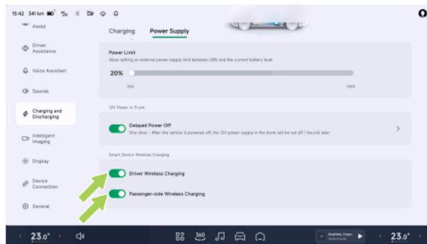
On the “→Charging and Discharging→Power Supply” interface of the CID, you can enable/disable the wireless charging function (if equipped) of front-row and second-row seats.
