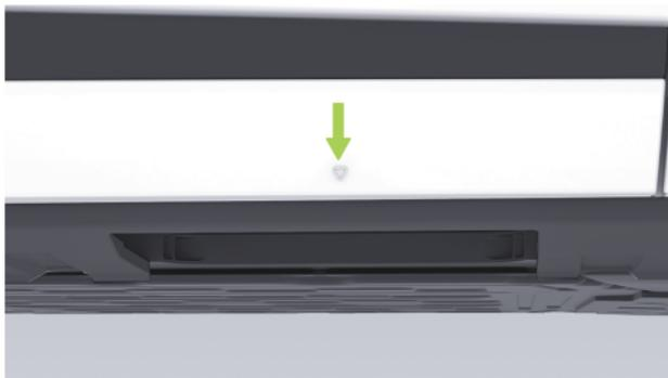
Vehicle lifting points can be identified by the arrows on the door lower trim panel.
