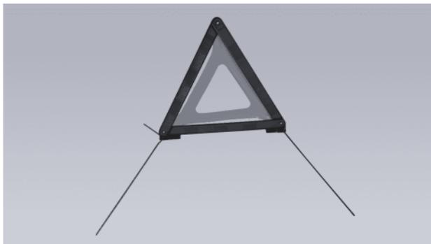
In the event of an emergency, remove the warning triangle, unfold it, and place it behind the vehicle. The placement positions are shown in the following table.
