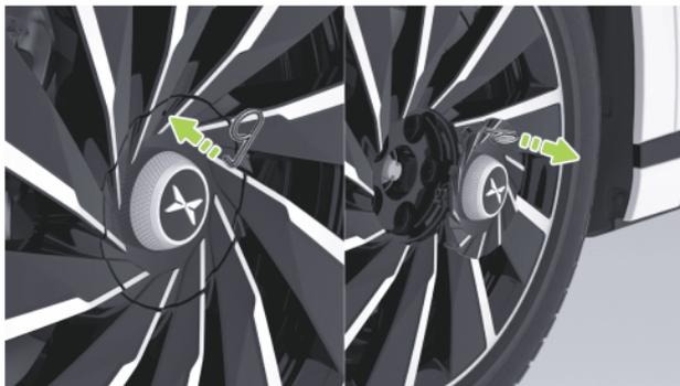
When replacing the tire, use the hook from the vehicle's tool kit. Insert it into the removal hole on the edge of the rim center trim cap, pull outward to remove the cap, store the hook back in the tool kit afterward, and keep it properly. During installation, align the rim center trim cap and press it hard until it clicks into place.
