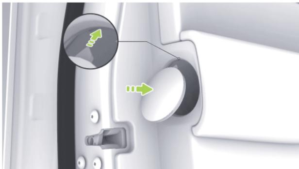
Insert the pin of the umbrella holder cover into the bayonet of the trim panel, and press the umbrella holder cover to reinstall it.
