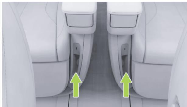
A mobile phone holder is set under the inner side of the second-row seat to hold a mobile phone.
