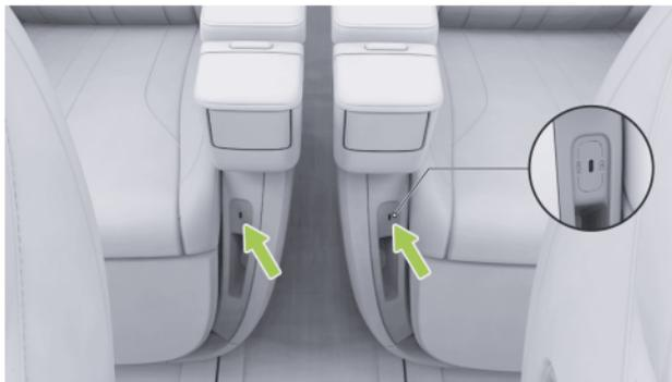
A Type-C power port is provided under the inner armrest of the second-row seat, with a maximum power of 60W.
