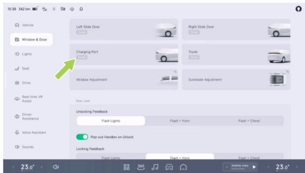
On the “**Window & Door**” interface of the CID, you can turn on/off the “**Charging Port**”.
