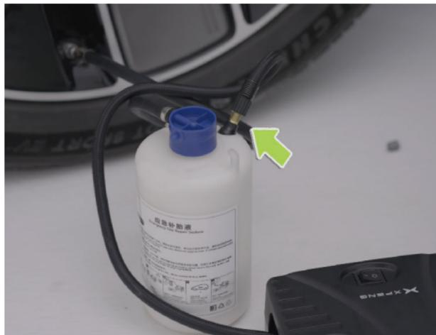
5. Connect the other end of the tire sealant hose to the air pump and tighten it, and connect the power cord of the air pump to the 12V power supply in the vehicle storage box.
