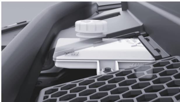
Check the level mark on the side of the brake fluid reservoir:
