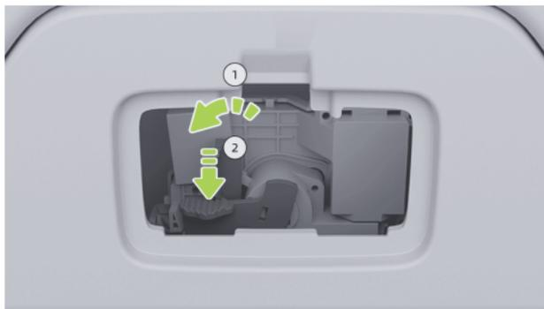
3. Pull the lever ① to the left and hold it, then press the lever ② to unlock the trunk, and then push the trunk outwards to open it in emergency.
