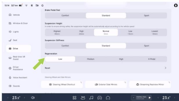
On the “**Drive**” interface of the CID, you can set different energy recovery levels.
