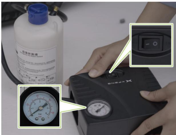
6. a. Turn on the switch to start the air pump, which will inflate the tire.
