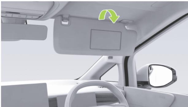
Sun visor can be flipped down in the direction of arrow to block sunlight coming in through front windscreen.
