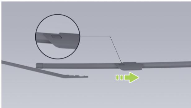
2. Lift the wiper arm, press the side locking button, and pull out the wiper blade to remove it.
