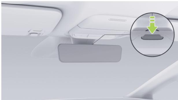
Press this button to switch from the streaming mode to ordinary mirror mode. Press the button again to switch to streaming mode.
