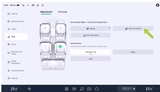
On the “**Seat**→**Adjustment**” interface of the CID, select a second-row seat, and tap “**Easy Entry/Exit**” to realize easy entry/exit.
