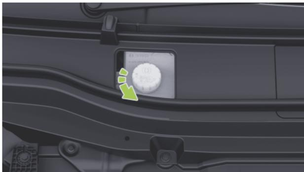
2. Unscrew and remove the reservoir cap.
