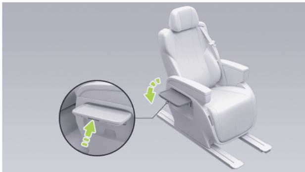
A foldable mobile phone panel is provided in the middle of the second-row seats for temporary storage of mobile phones. When it is not in use, press and hold the switch below the outer side of the panel to retract the panel.
