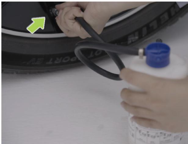
4. Screw one end of the tire sealant connecting hose tightly onto the tire valve. Ensure the sealant container is not inverted.
