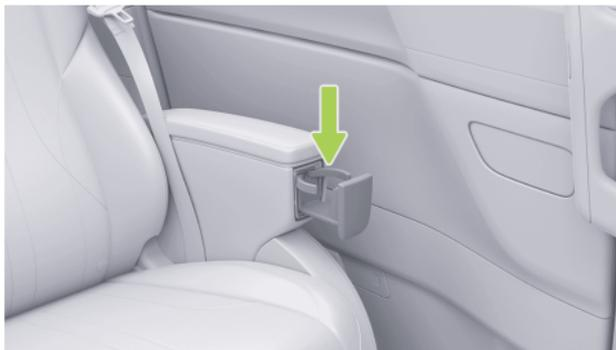
The outer armrest of the second-row seat is equipped with a cup holder to hold drink bottles or cups. It can be pulled out when in use and pushed back when not in use.
