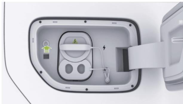
Charging port cover can be closed by pressing the switch.
